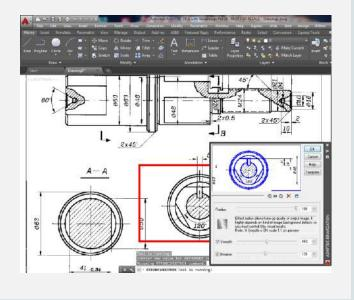
In WiseImagefor AutoCAD tools it is possible to crop, change resolution, scale, deskew, and calibrate colour and greyscale raster images. It is possible to change brightness, contrast, hue and saturation and adjust the colour gamut, improve image quality and apply colour. Users can rasterize vectors to generate ISO compliant raster as often required for compliancy purposes. Merging monochrome and colour images is also a one-click task.
